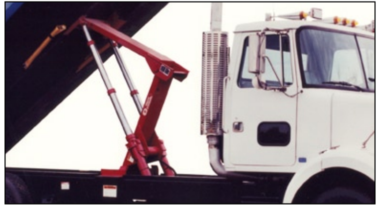
The 144 HD Hoist shown mounted with the hinge forward (Black paint standard)
